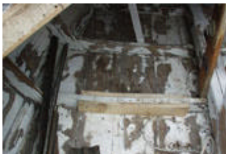
What's wrong with this picture? Splints, or replacement "sister" frames used to strengthen cracked frame
