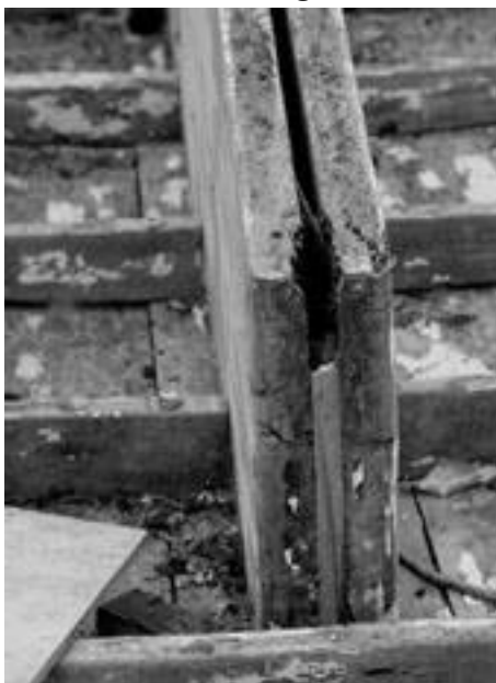
Rotten centerboard trunk with crudely glued repair stick at sternmost end
