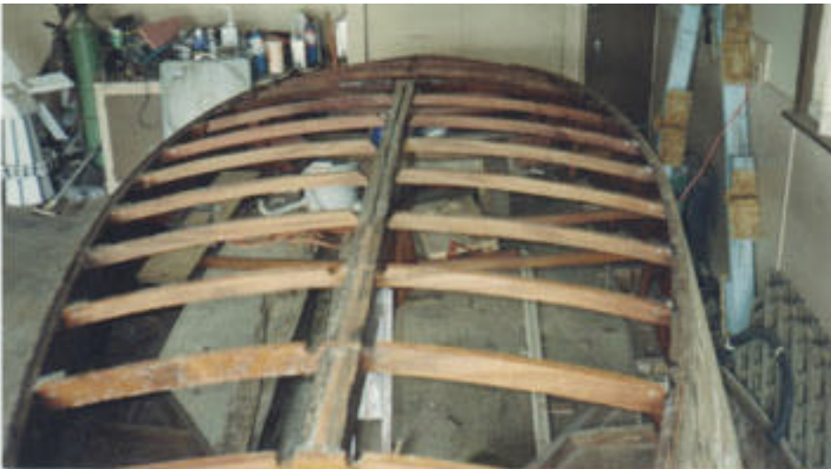
New ribs installed and cedar planking reinstalled
