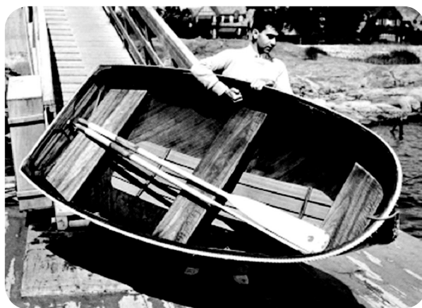
Figure 6. Molded mahogany Hydrolite dingy. Note the veneer pattern what we see in wooden Thistles
